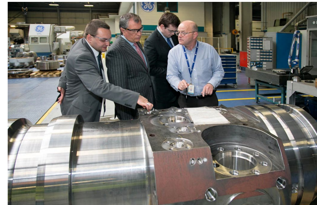
General Electric specialists demonstrate components of underwater wellhead equipment. The equipment is used for the sealing of offshore wells
